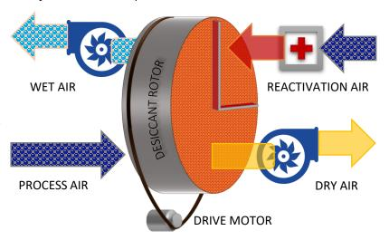
AAI's desiccant dehumidifier can achieve ultra-dry-air at any desired application temperature requirement. NSI-D series is suitable for continuous operation as the dehumidification process is condensation free.
